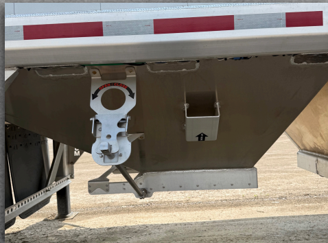
Self locking chute opener & hammer hit bracket
