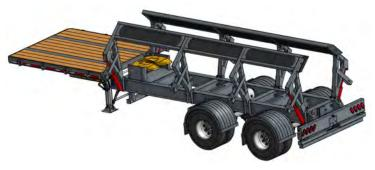
Tandem Pup Verison Shown w/ No Aluminum Chemical Cabinet Sprayer Fifth Wheel Plate Lock Option Shown Hydrualic Fold Option - Folded Position
